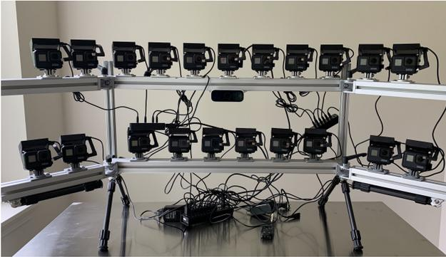
Figure 2. **Our multi-view capture setup** using synchronized GoPro Black Hero 7 cameras.
